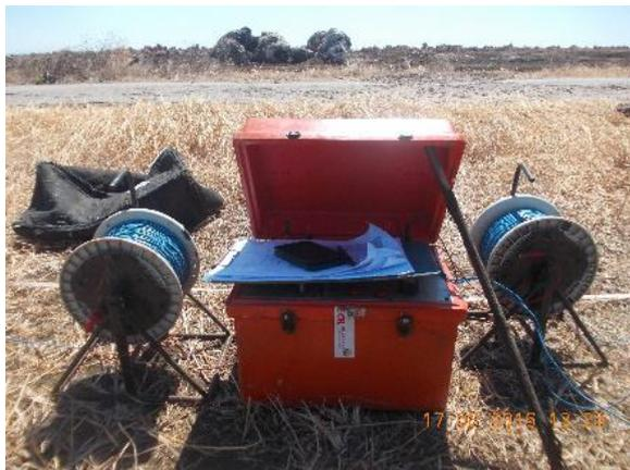
**Figure 4.** Electrode planting Schlumberger method
