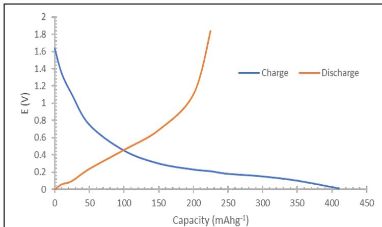
The charge and discharge capacity obtained from coal sample of B 106-crb are 418.4, and 225.3 mAh g<sup>-1</sup>, respectively. The Initial Coulombic efficiency (ICE) is 53.8%.
