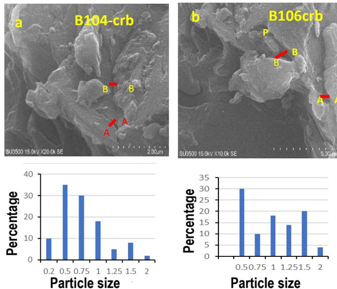
The micro-fissures and micro-pores of coal samples B 104-crb and B 106-crb have been determined by SEM analysis. The B-104-crb has a micro-fissure aperture smaller than in B-06-crb) are 0.25 nm and 0.55 nm, respectively. The coal sample of B 106-crb is more porous than B 104-crb.
