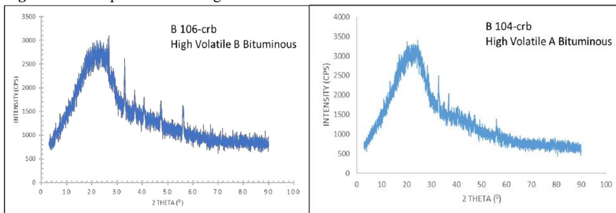
The coals are characterised by having a high diffraction peak (002) and narrowed diffraction peaks (002). Calculation of the interlayer spacings of carbon hexagons ( $d_{002}$ ) of each coal was also relatively similar (Table 3).
