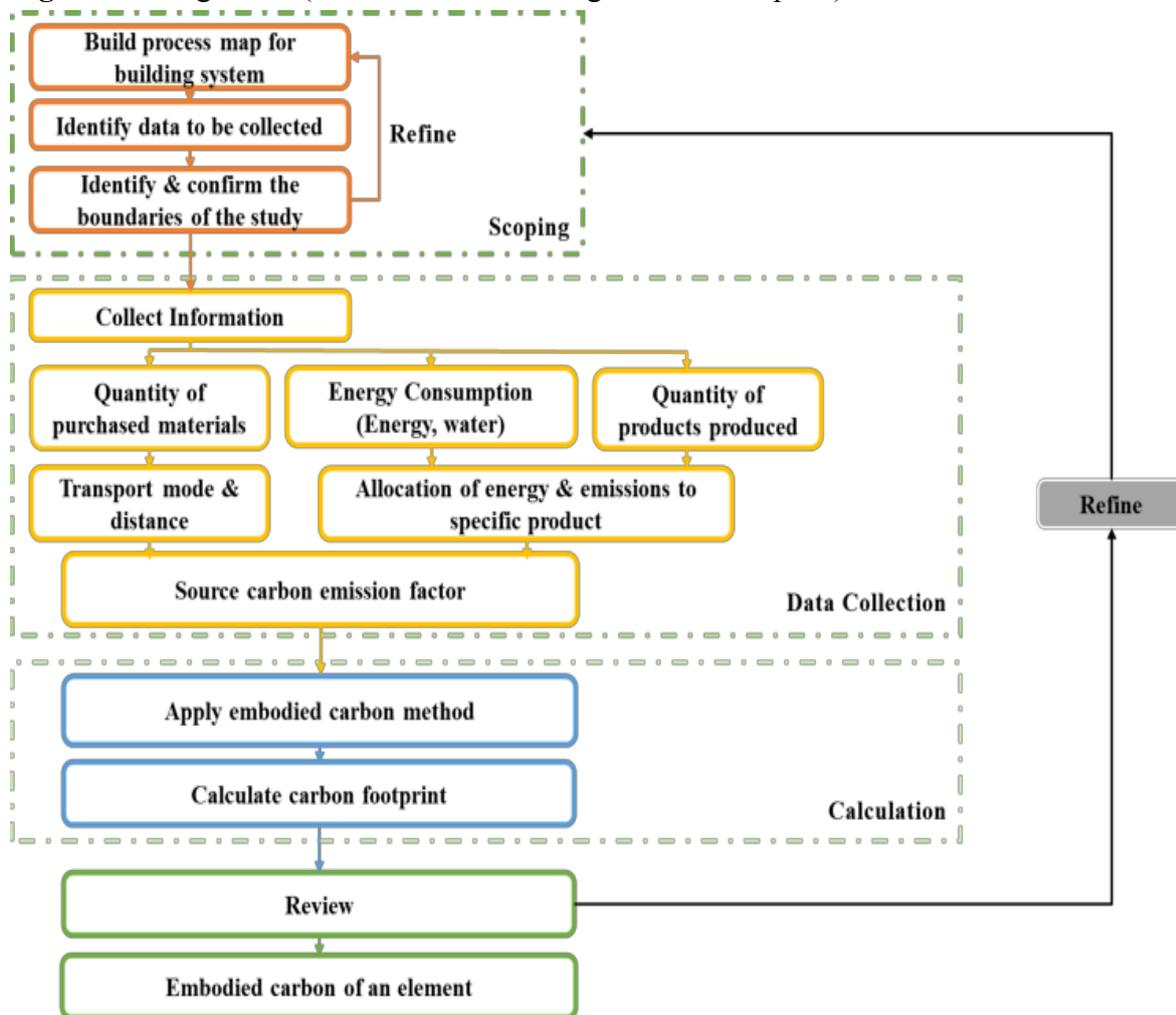
The integration of BIM into LCA has great potential to compute carbon footprints over its project life cycle. It aids QS in determining the environmental impact of building materials when selecting them. The finalized framework is based on analysis and comprehensive discussion, as well as inputs obtained through both preliminary research and structured interviews. However, this model is yet to be validated and further research is highly recommended.
