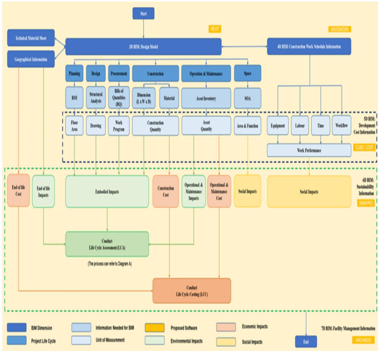
The finalized BIM-enabled LCA framework is as Figure 4 and Figure 5. It was developed based on ISO 14040:2006 and Royal Institution of Chartered Surveyors (RICS) professional standards and guidance as to whole life carbon assessment, for built environments, to develop an LCA framework with a proper input and understanding. The LCA framework was then mapped onto the digital construction process using BIM as a platform.
