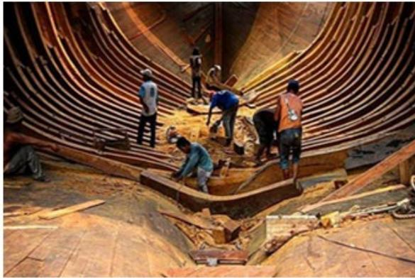
(a) Body Construction of Pinisi Vessel
