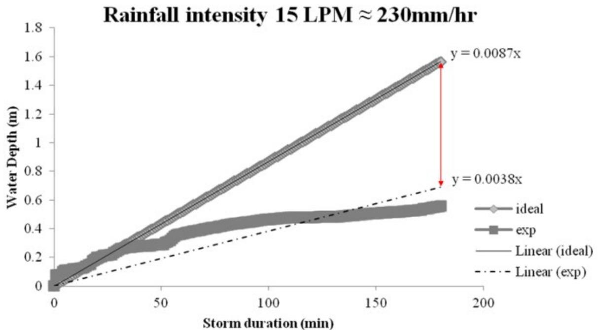
All the processes are deliberately organised to happen in order to see any possibility of water losses. Therefore, three different rainfall intensities are used on the similar CDP system in order to see the movement of water if the subgrade state is not in a fully saturated condition. The water budget concept was applied to this situation.
