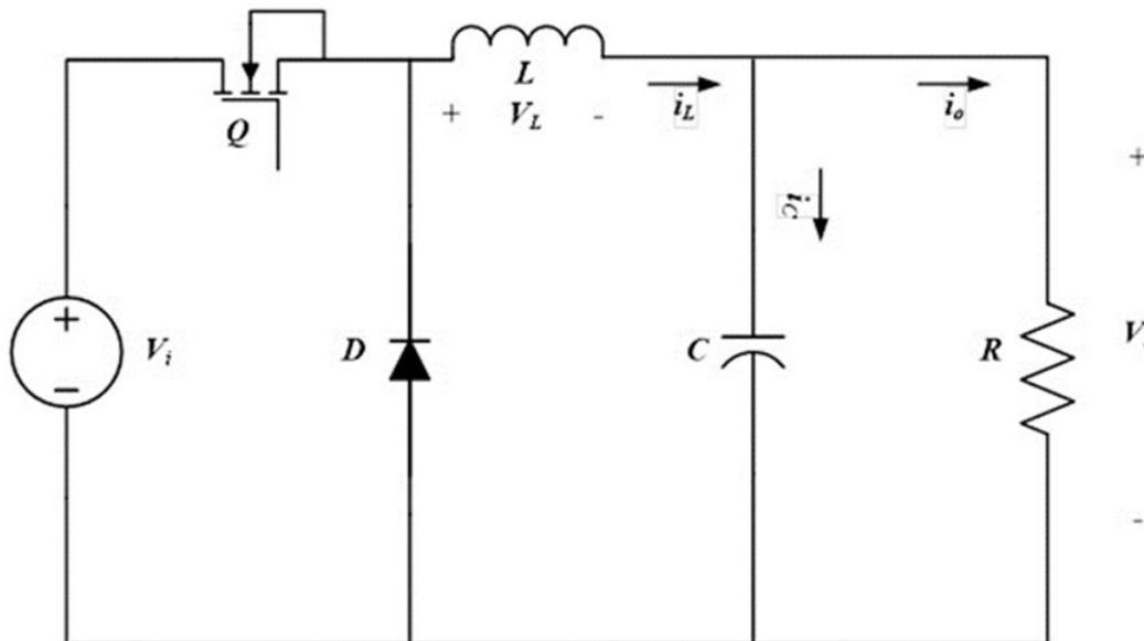
**Figure 3.** A prototype of Buck converter circuit
